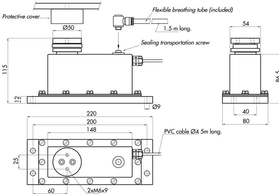
**DIMENSIONS LOAD CELL MODEL 260 50÷200 KG CAPACITY**
