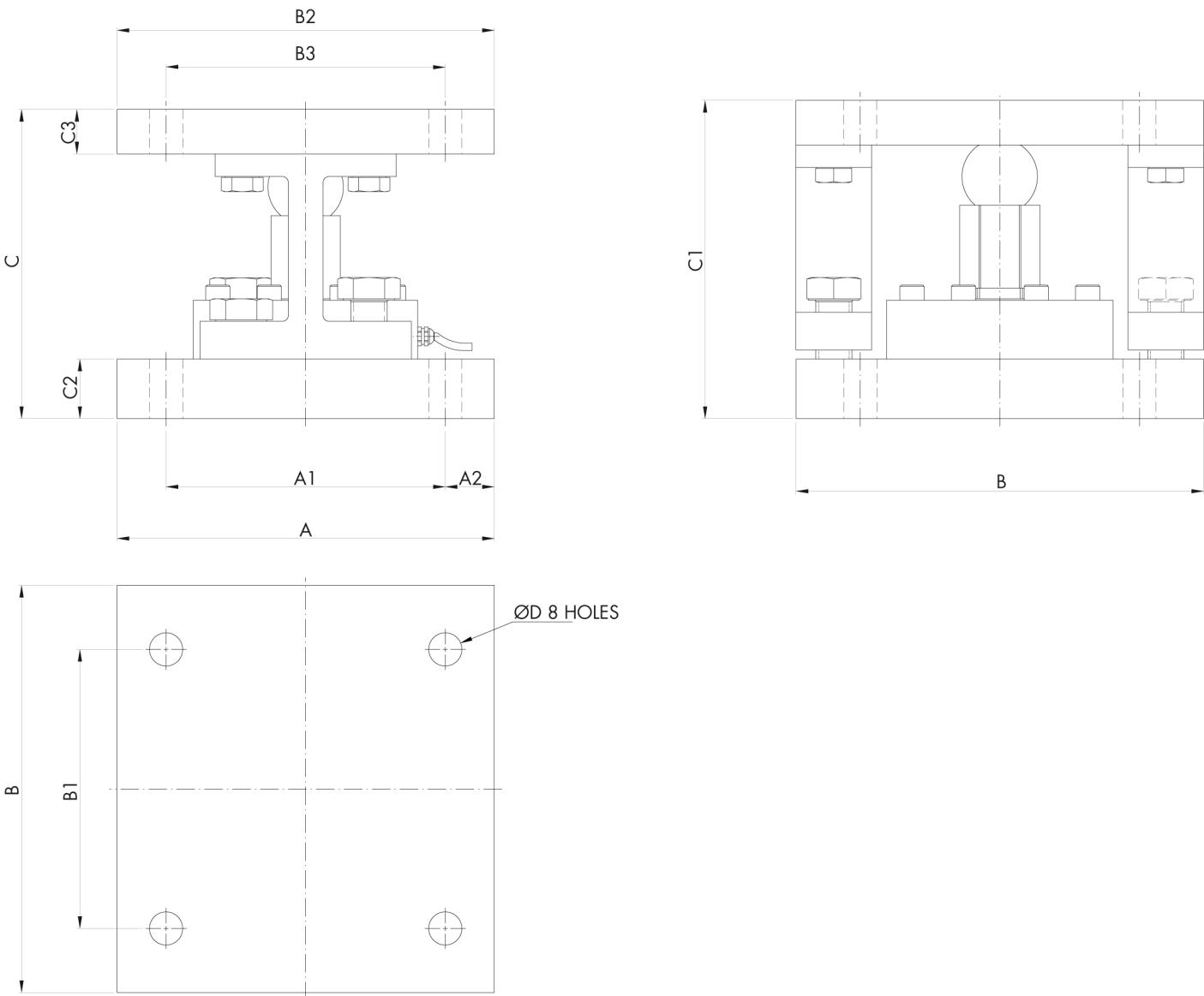
**ALLOY STEEL (capacity, dimensions and maximum load values by model)**
